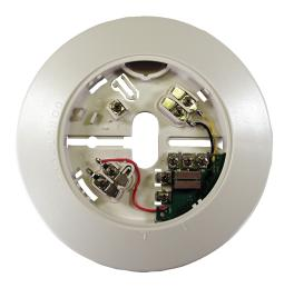
The F220-B6 Series Detector Bases work with the F220 Series Photoelectric Smoke and Heat Detectors. The F220-B6 is a 12 V or 24 V base for two-wire loops. The other bases in this series are 12 V or 24 V bases for four-wire loops.
